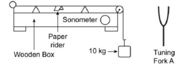
The diagram above shows a wire stretched over a sonometer. Stems of two vibrating tuning forks A and B are touched to the wooden box of the sonometer. It is observed that the paper rider (a small
