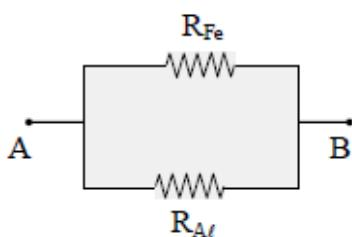
$$R_{fe} = \frac{\rho \times 50 \times 10^{-3}}{(2 \times 10^{-3})^2} = 1250 \text{ ohm}$$
